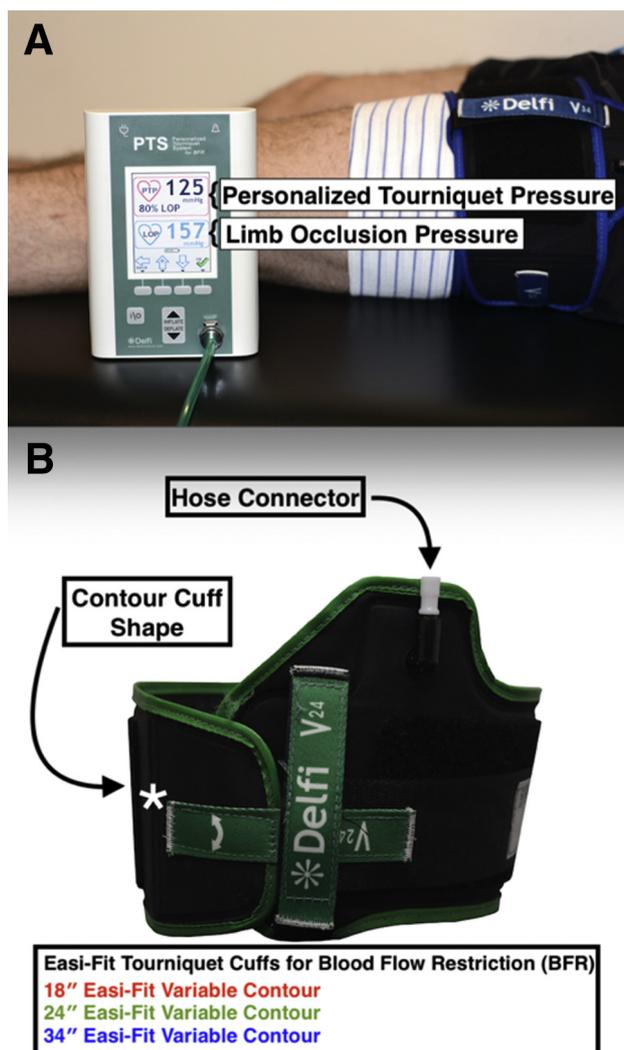
**Fig 2.** The components of blood flow restriction (BFR) consist of a personalized tourniquet system (A), which tailors the personalized tourniquet pressure to each patient after determination of the limb occlusion pressure, and a contoured tourniquet cuff (B), which is available in 3 different lengths (length use is dependent on patient thigh size). These components are then connected by a hose assembly. \* indicates the contoured strap of the personalized tourniquet.
